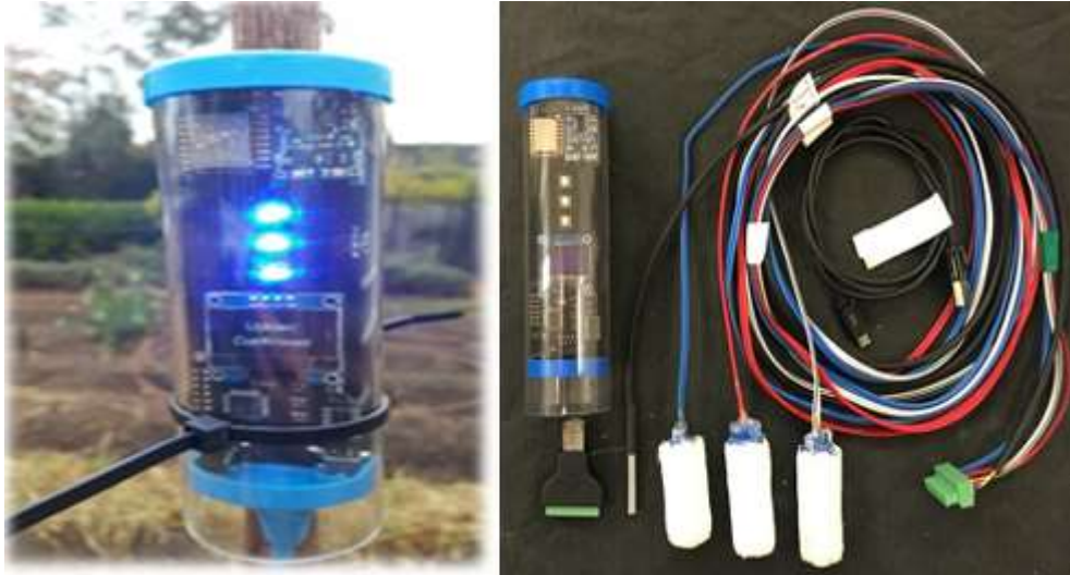
Figure 1 Chameleon wi-fi field reader and set of sensor arrays
