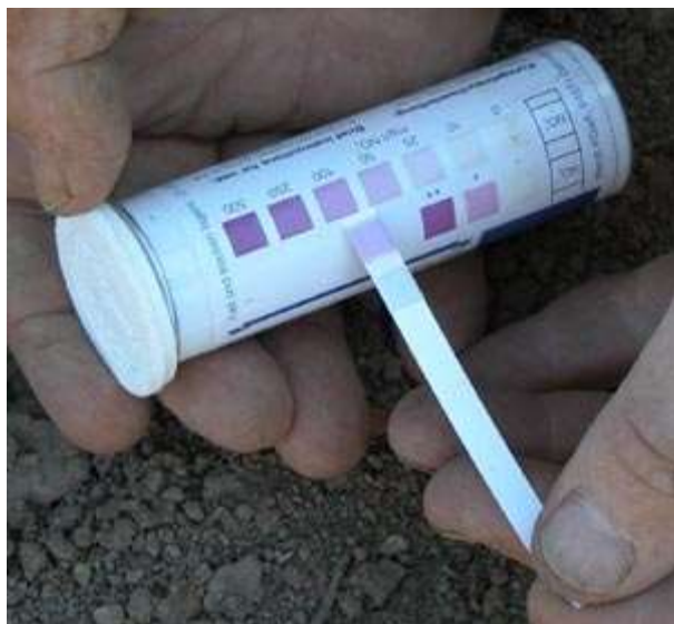
Figure 3 Nitrate strip (4a) and Chameleon EC meter (4b) used to show how much nitrate is there within a particular soil depth and electrical conductivity respectively
