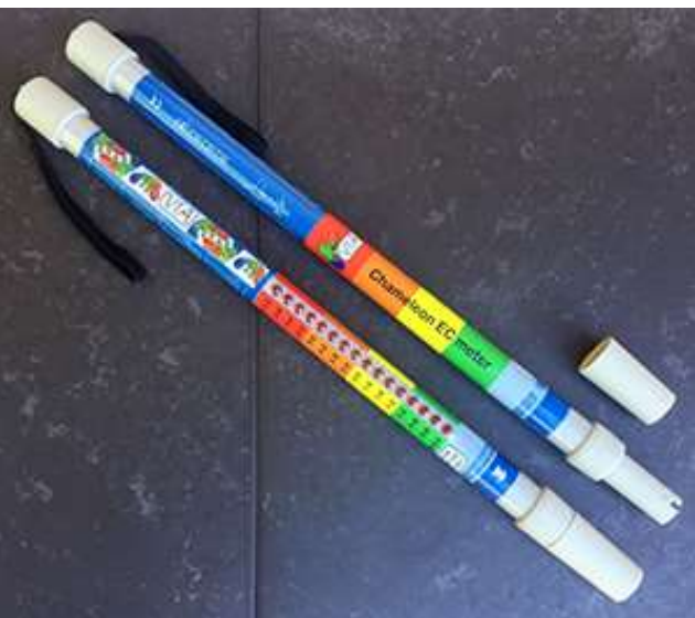
Figure 3 Nitrate strip (4a) and Chameleon EC meter (4b) used to show how much nitrate is there within a particular soil depth and electrical conductivity respectively
