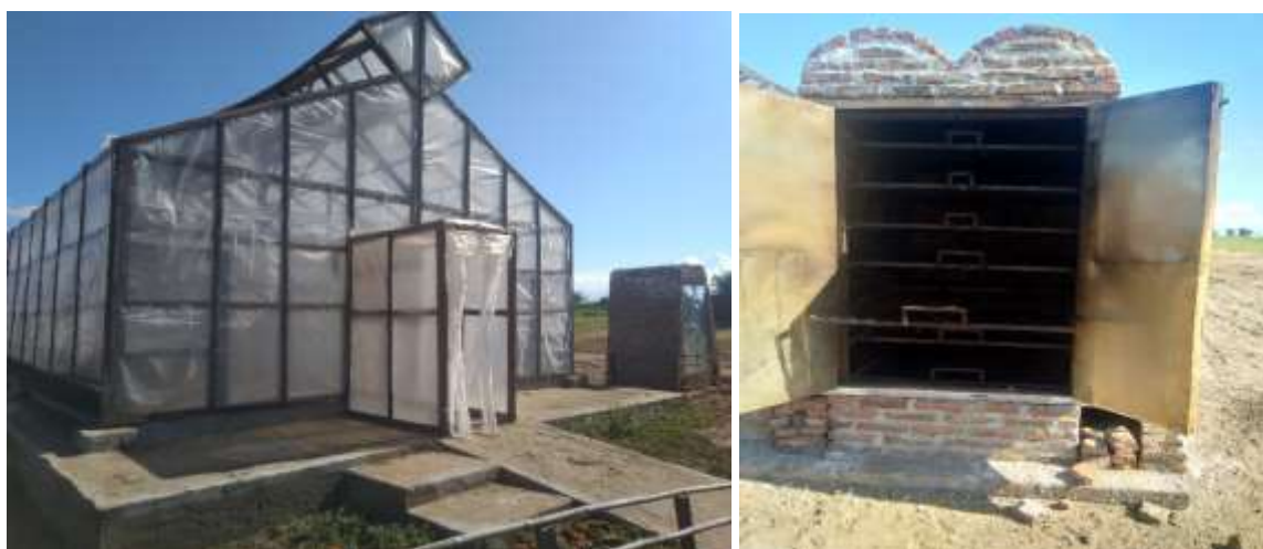
Figure 11 Personal solar tent drier and improved smoking kiln at Malembo
